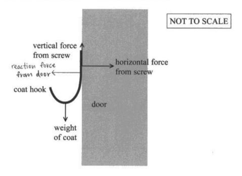
Add a labelled arrow to the diagram to show the additional force required for the coat hook to be in equilibrium.
